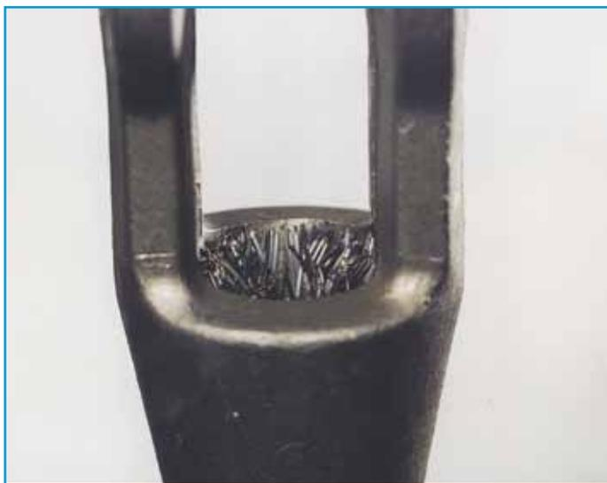
Properly positioned broom with the wire ends protruding slightly (Fig 3)
