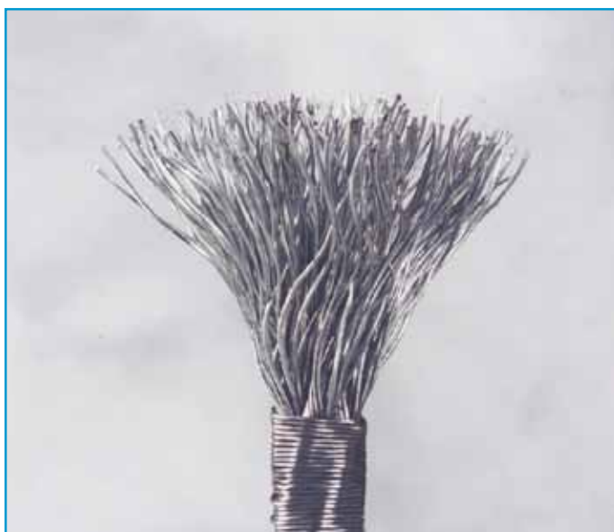
Properly Broomed Wire Rope (Fig 2)
