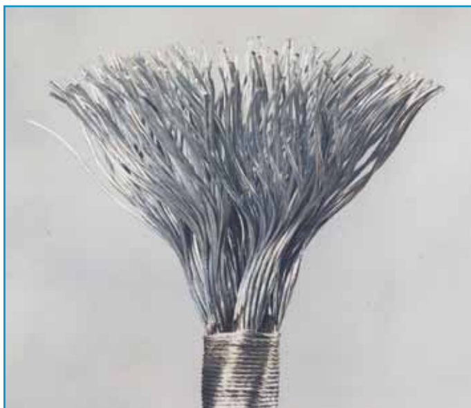
Incorrectly Broomed Wire Rope
