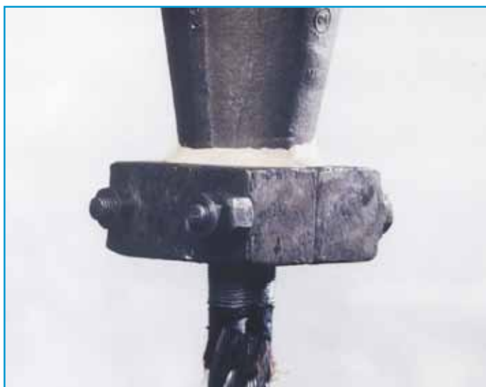
Clamp used to align rope and socket before sealing with plasticine (Fig 5)
