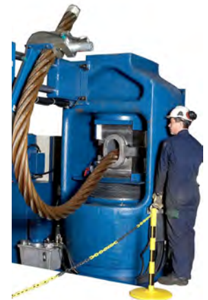
RBS mounted on a swager
